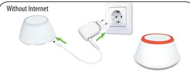
f you are installing an underfloor system without an Internet connection, you can use the coordinator from the KLO8RF instead of the Universal Gateway.
